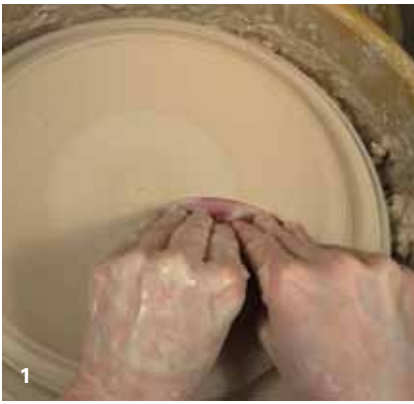
1 Use a rib to shape and smooth the center of the plate.
